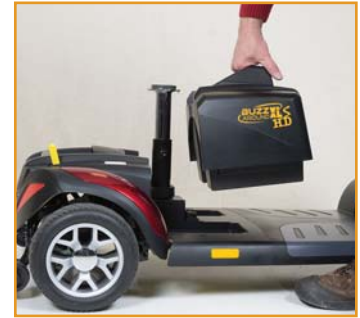
Step 2: Pull out the battery pack!
