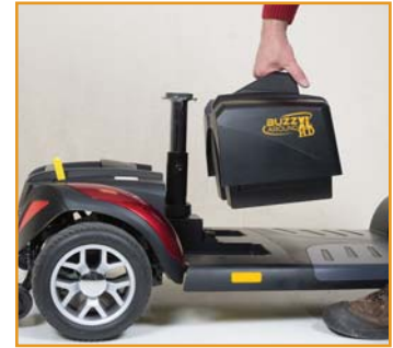
Step 2: Pull out the battery pack!
