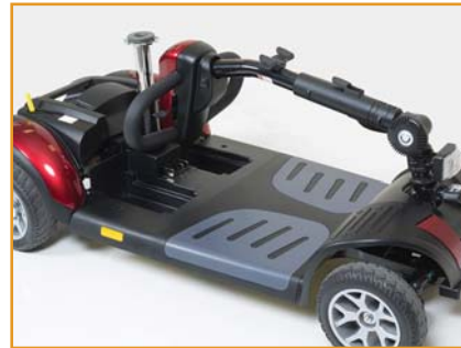
Step 3: Fold down tiller and lock in place!
