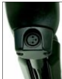
Charger port relocated under controller
